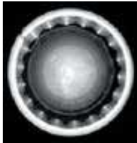
Broken Tamper Band
